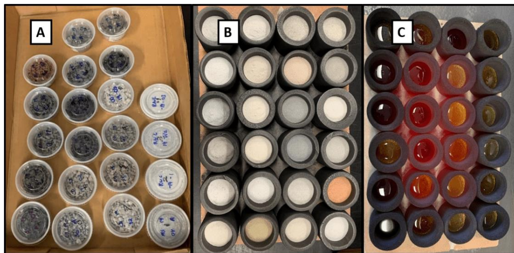
Figure 7: XRF and ICP-MS geoanalytical process conducted by Chanel Dvorak at Washington State University, Pullman Campus. (A) Rock chips were brought to WSU from PSU in the process of crushing rocks to powders. (B) Round two of crushing rocks into powders at WSU and post addition of dilithium to powdered samples and placed in carbon crucibles. (C) Samples were cooling into beads from being melted in an oven at 1000^\circ\text{C} . Further processes are conducted to generate XRF and ICP-MS data.
