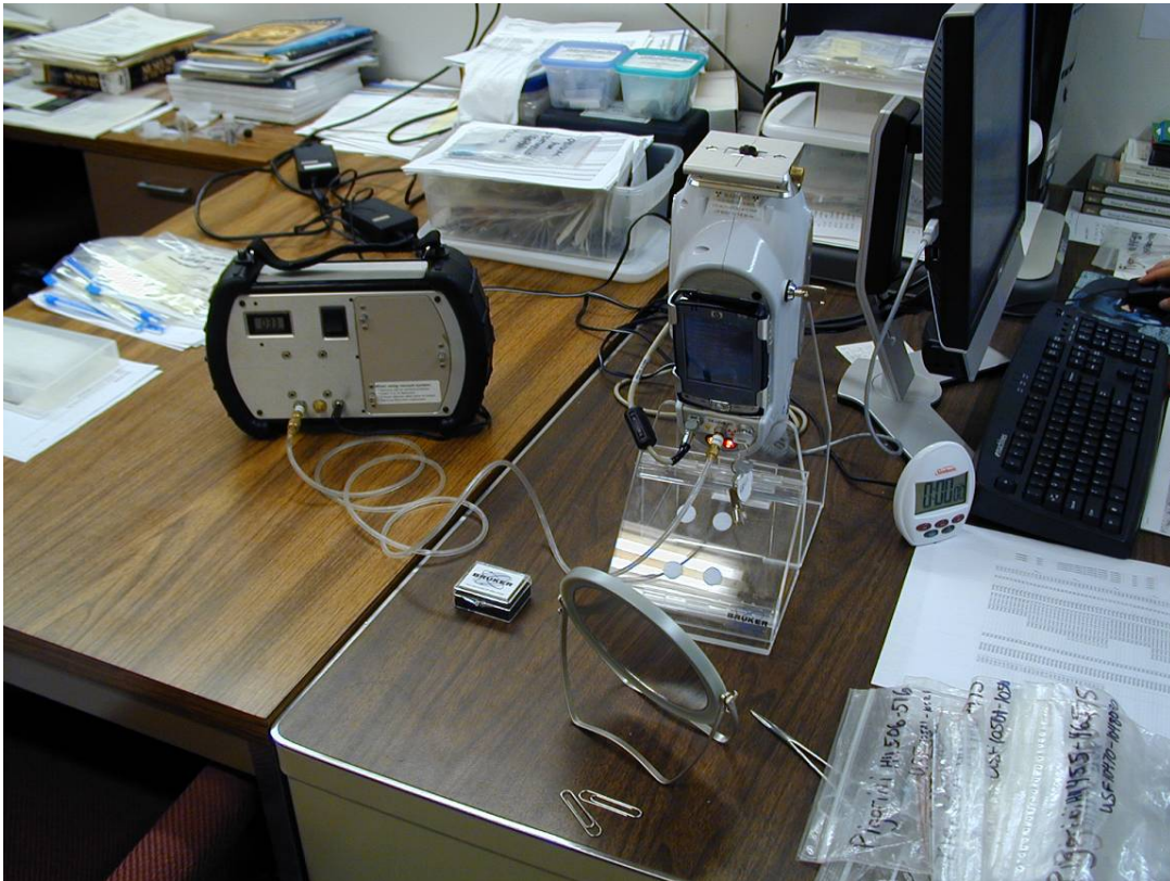
Figure 4.3. A Bruker Tracer III-V portable XRF machine (photo by Robert Tykot)
