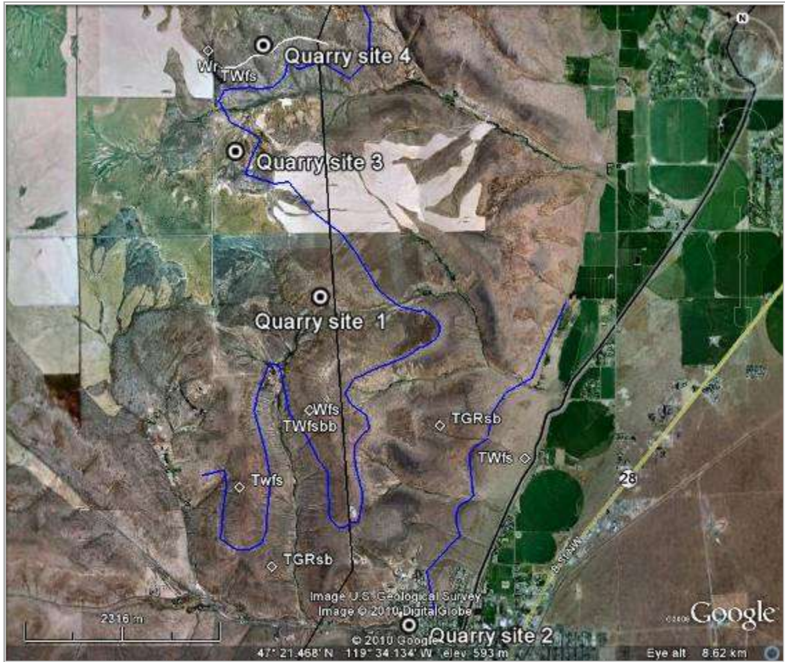
Figure 5.7 Location of five Beezley quarry sites. TWfsbb is Frenchman Springs Babcock Bench flow; TGRsb is Grand Ronde flow. Generalized stratigraphy is based on previous work by Le Fervre, (1967); Grolier and Bingham (1971, 1978) and Swanson et al. (1979a), who identified the local basalt units and their distributions. The basalt contacts were mapped in the field for this dissertation project, and transferred to the air photo.
