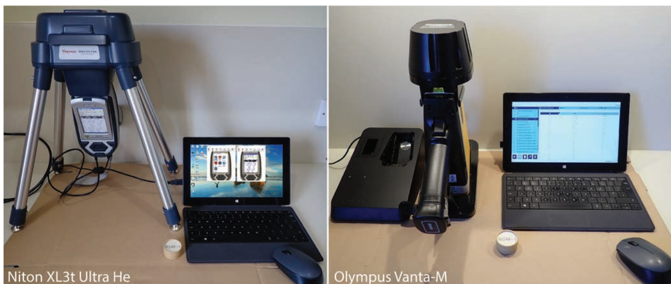
Figure 4. The pXRF analyzers used for chemical fingerprinting and source characterization of the Late Neolithic obsidian assemblage from Hódmezővásárhely-Gorzsa (photographs by C. Bonsall).
